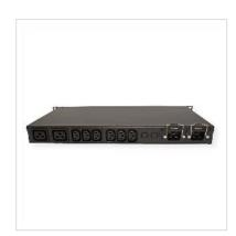
The Automatic Transfer Switch (ATS) is a high availability device designed for providing redundant power for sensitive electronic equipment. Powered by two independent power sources, it makes a rapid switch from one source to the other automatically, when the power supply used to power its connected load fails.
